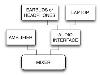
Monitors, speakers, laptop, audio interface, and microphones, if desired (not needed), are connected by cables to the mixer, which is usually centrally placed in the back of the auditorium, or otherwise, on the side of the stage.
